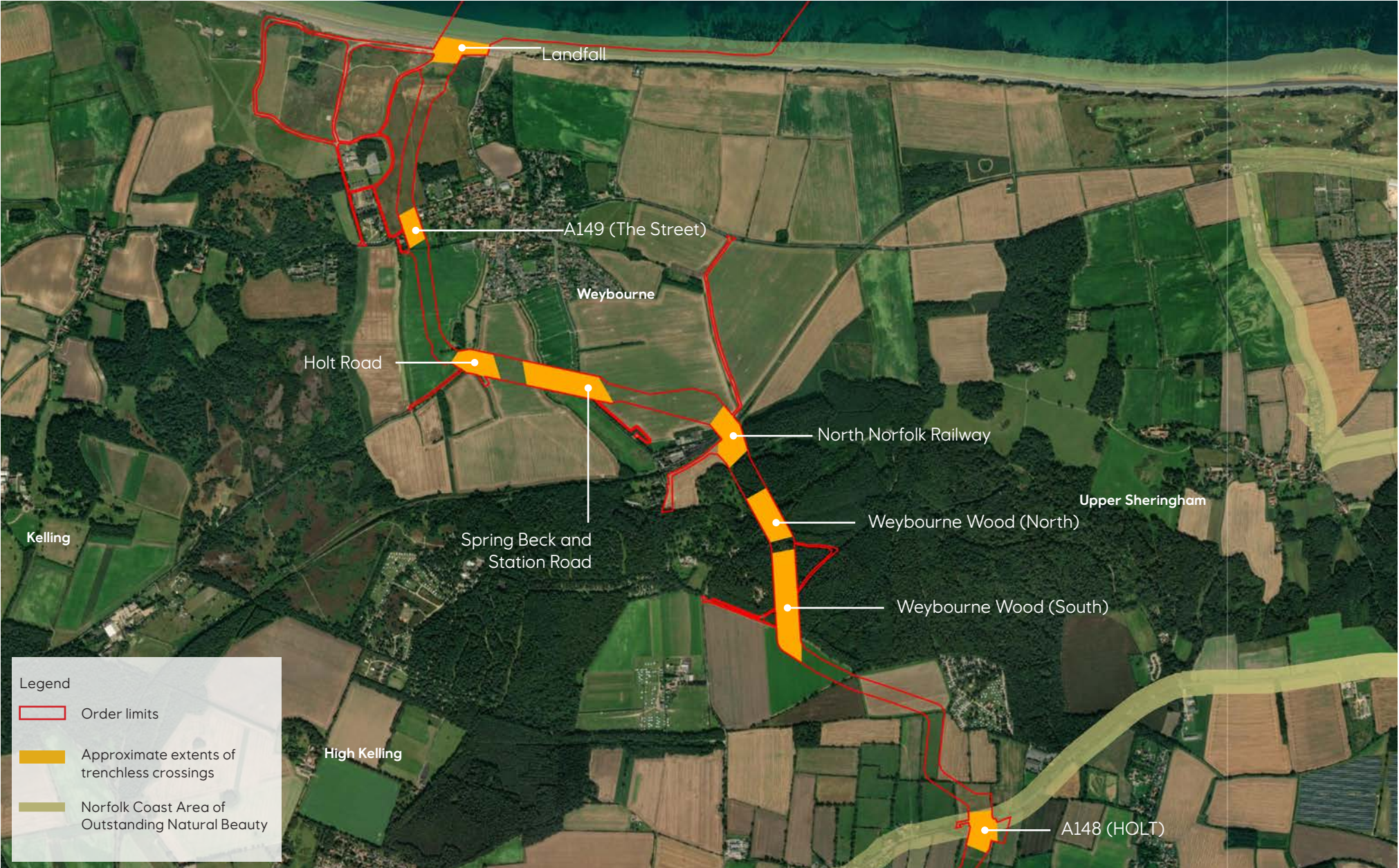
FIGURE 6.3: Approach to cable routing through the AONB [updated]
