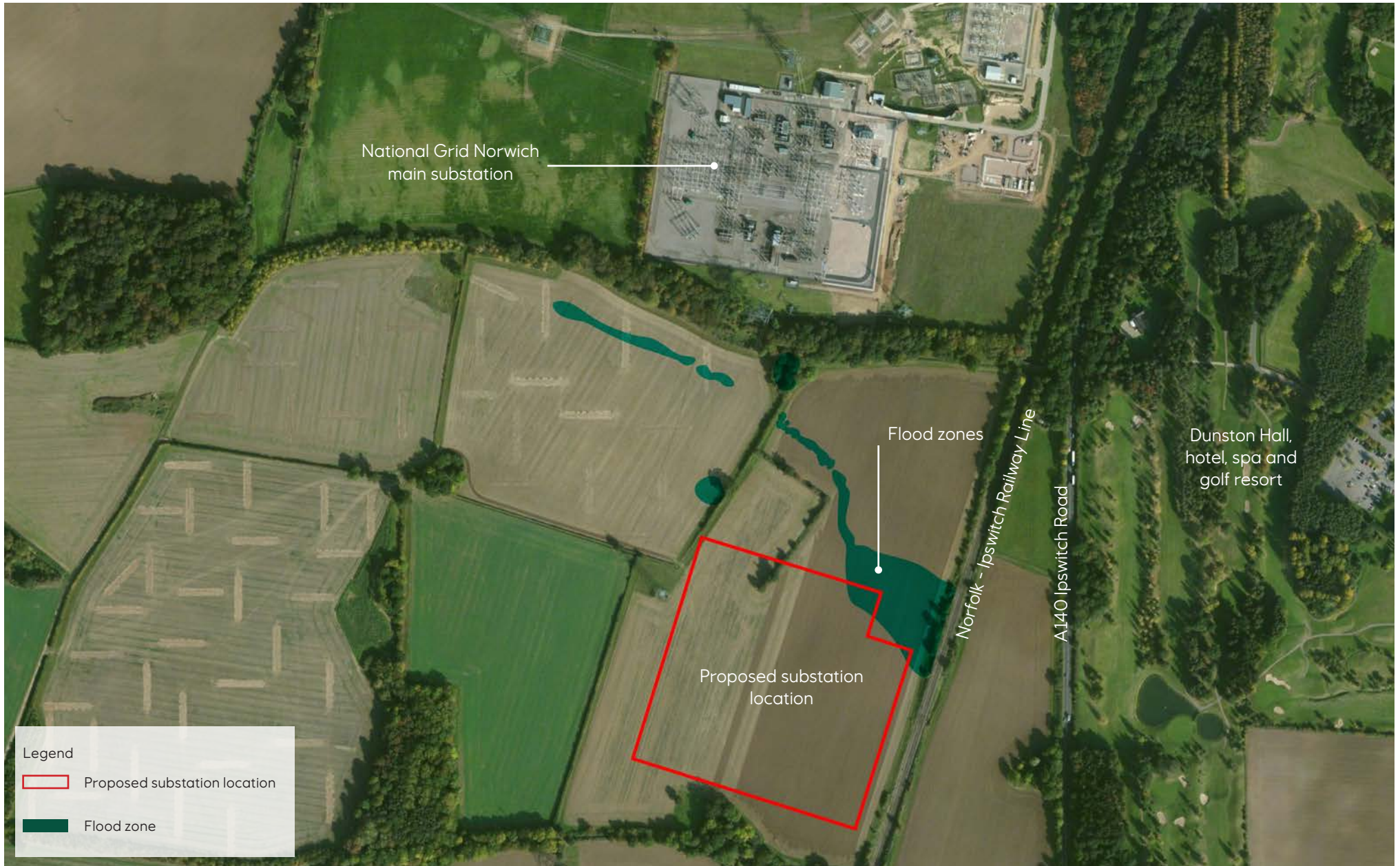
FIGURE 7.1 : Substation location and flood zone
